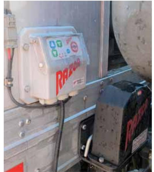
The Razor Top Runner power tarp easily operates via the switch behind the cab, or a wireless remote, and takes less than 60 seconds.
