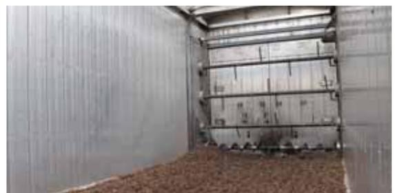
Inside the almost empty body, with the walking floor feeding the mulch into the levelling bars and rear augers and dropping into the blower motor.
