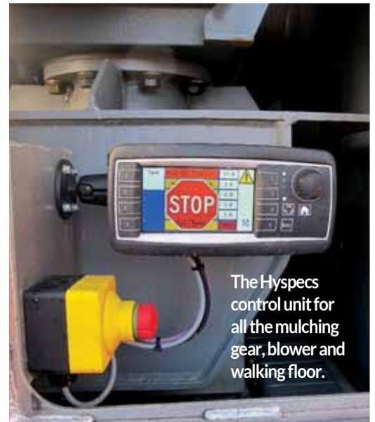
The Hyspecs control unit for all the mulching gear, blower and walking floor.
